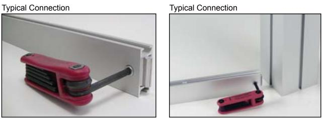
Detail A: Most horizontal extrusion connections have a patented expandable lock. This lock inserts into the groove of an opposing extrusion. Tightening the lock with the Hex Key Tool expands the lock and creates a strong positive connection.
