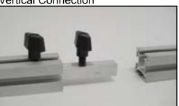
Detail E: A square connection bar with plastic T Knobs is inserted between two vertical extrusions joined end-to-end. Turn the knobs clockwise to tighten. Do Not Overtighten.
